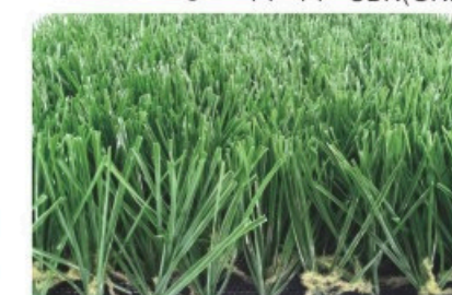
SHA-23418 Type: DSU62-5016 Pile height: 50 mm Stitch Rate: 16 /10cm Gauge: 5/8 inch Density: 10080 stitches/m 2 Dtex: 6200 Backing: PP+NET+SBR
