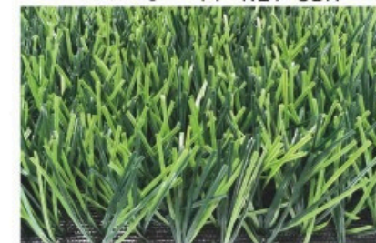
SHA-23420 Type: PRO-2-5016 Pile height: 50 mm Stitch Rate: 20 /10cm Gauge: 5/8 inch Density: 10080 stitches/m 2 Dtex: 8800 Backing: PP+NET+SBR
